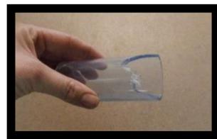
When drilling holes in PVC, start with a small drill bit to make a pilot hole. Then use a bit a few sizes larger and enlarge the hole. Continue using increasingly larger bits until you reach the hole size you desire. Drilling holes in the clear PVC makes some large burrs, but they are fairly easily removed with the blade of your pocket knife.
