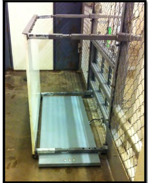
**Figure 16** - A side view of the chute with the scale in place. The scale slides right under the bottom "C" bars.
