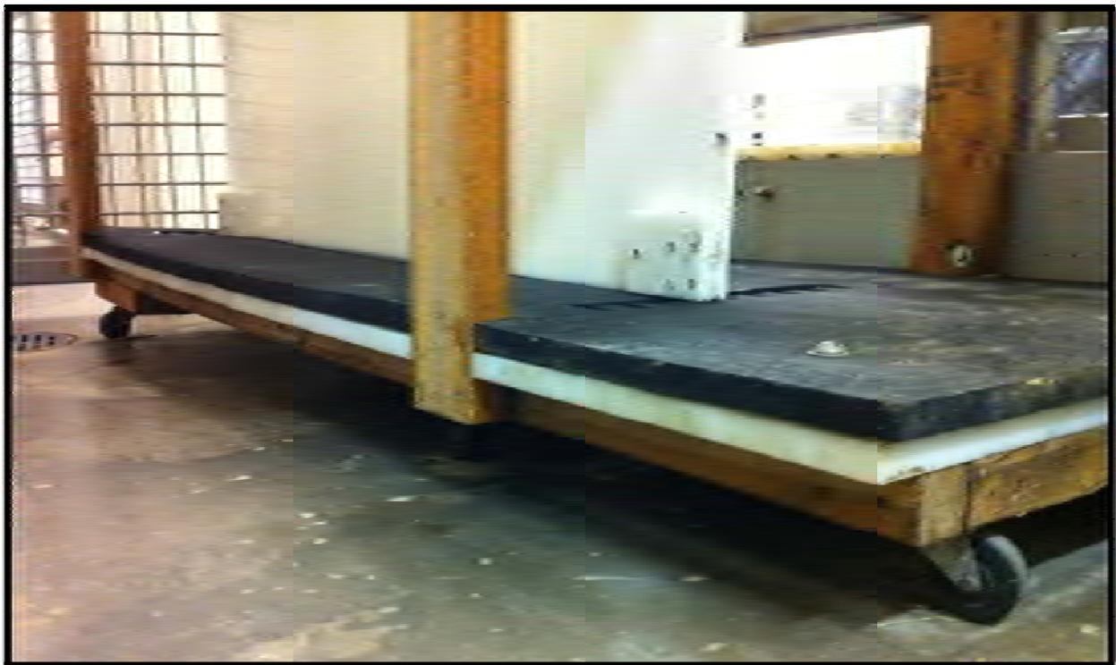
**Figure 3** - This shows the base of the chute with the layers of the wood frame, HDPE, and the rubber mat on top. There were six wheels spaced out along the bottom for mobility.
