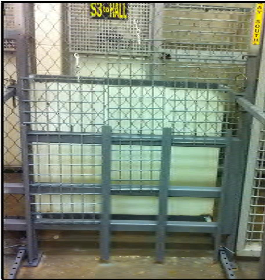
**Figure 14** - This shows the new bottom openings that were created and all the different possible openings that can be exposed for husbandry or medical needs. The left bottom opening is to access feet. The middle opening is to access the belly. The right top is to access the hips.
