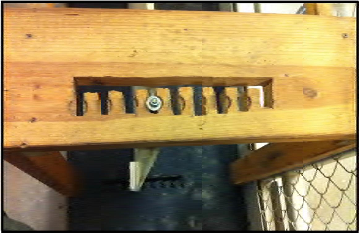
**Figure 6** - This is a top view of the notches that allowed the back wall to move forward and backward and lock in place.
