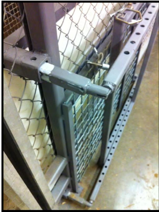
**Figure 11** - A top/side view to show how condensed the chute is when it is closed and not in use. The hinges used in the design are also seen.
