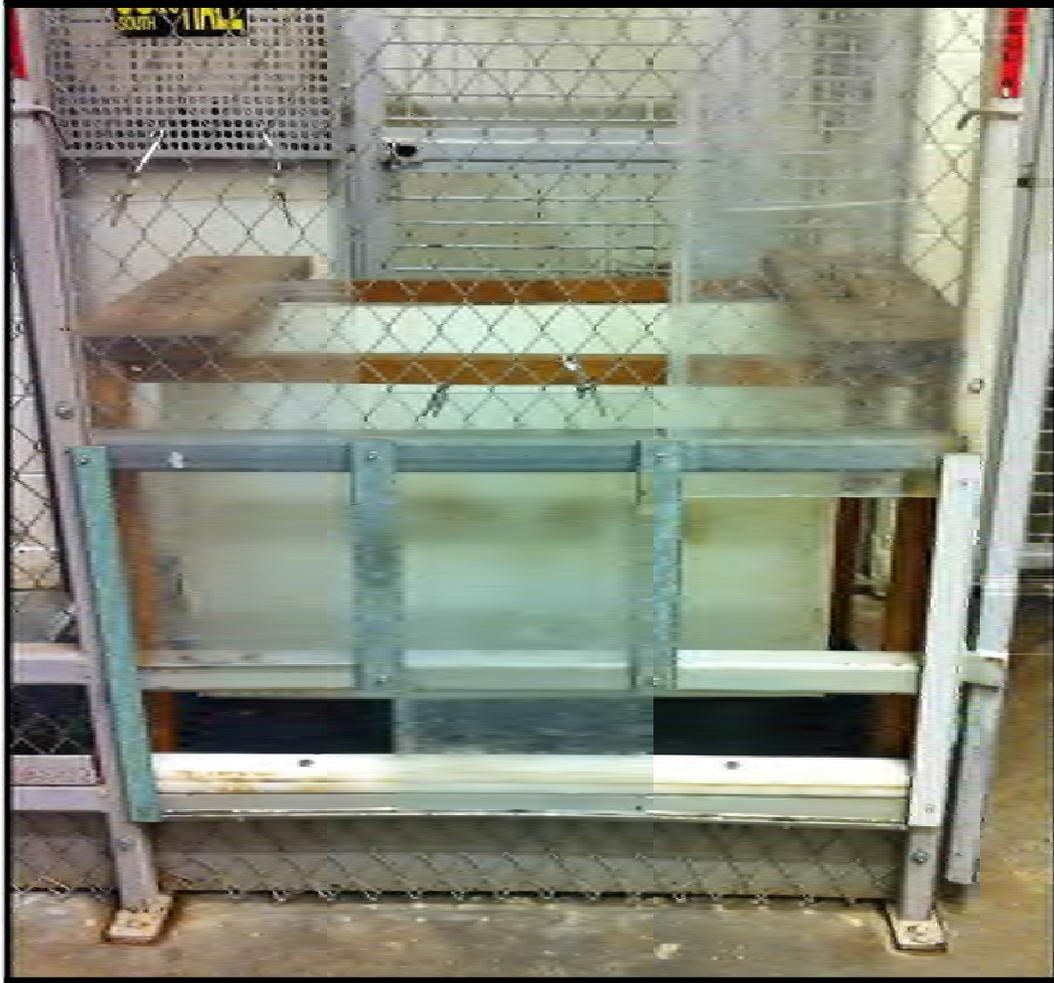
**Figure 2** - This shows two of the Plexiglas® panels slid upward and clipped in place to expose different openings. In this picture, the left bottom hole is where the hog would be fed. The top right opening is where the hip would be exposed to perform different behaviors.
